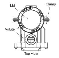
**WARNING** - If the pump is being pressure tested, release all pressure before removing trap cover. Do not block the pump suction while the pump is running. If a body part blocks the pump suction it may cause severe or fatal injury. Small children using the pool must ALWAYS have close adult supervision.
