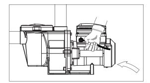
4. Reinstall the RS-485 communication cable.
